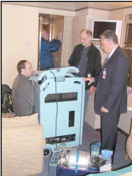
The ViroForce ozone generator/catalytic-scrubber prototype and the rapid humidifier prototype were placed on the floor within the cabin as shown in the photo to the left. Room vents were sealed off with duct tape to prevent any ozone from escaping the cabin. The cabin dimensions were measured and the cabin volume was calculated to be 1308 cubic feet.
